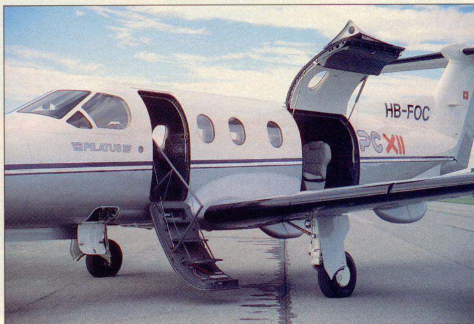
An airstair door for the passengers, a gaping maw for the cargo. Closing the cargo door is a matter of hitting a belly-mounted push button. Battery power then lowers the door to the locking position.
